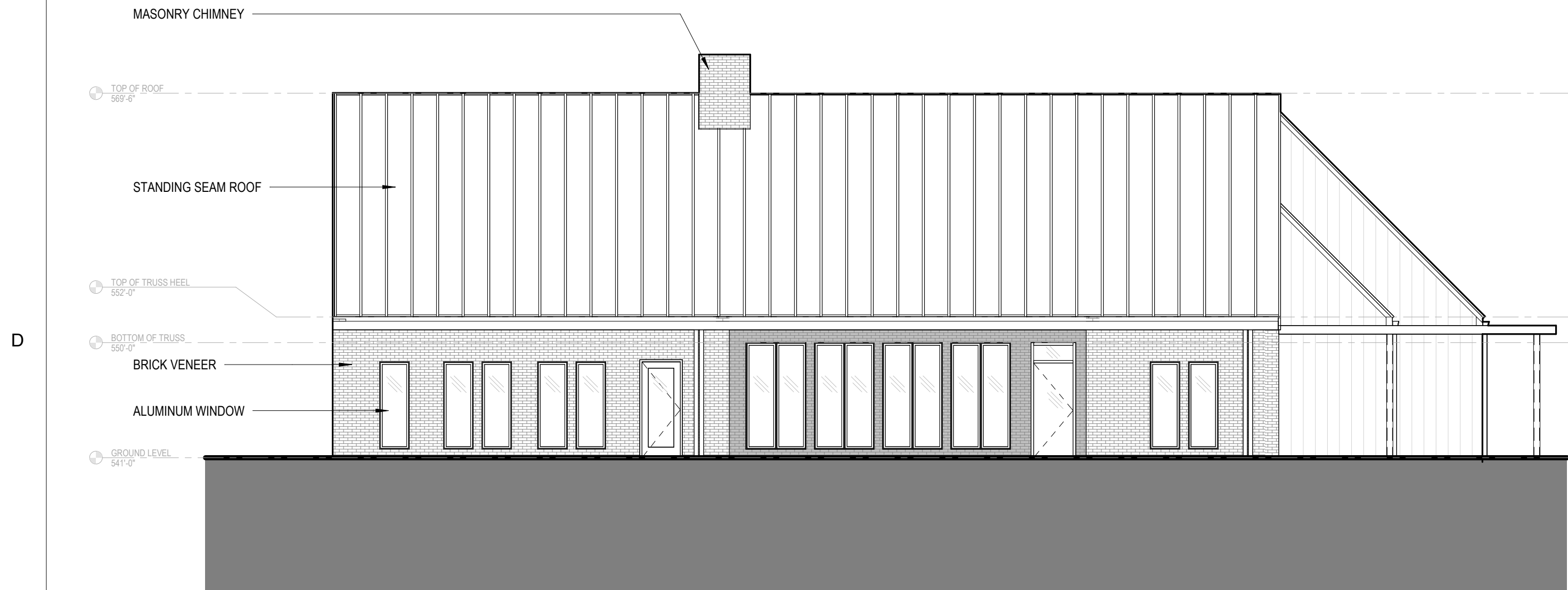
D1 EAST BUILDING ELEVATION 1/8" = 1'-0"
