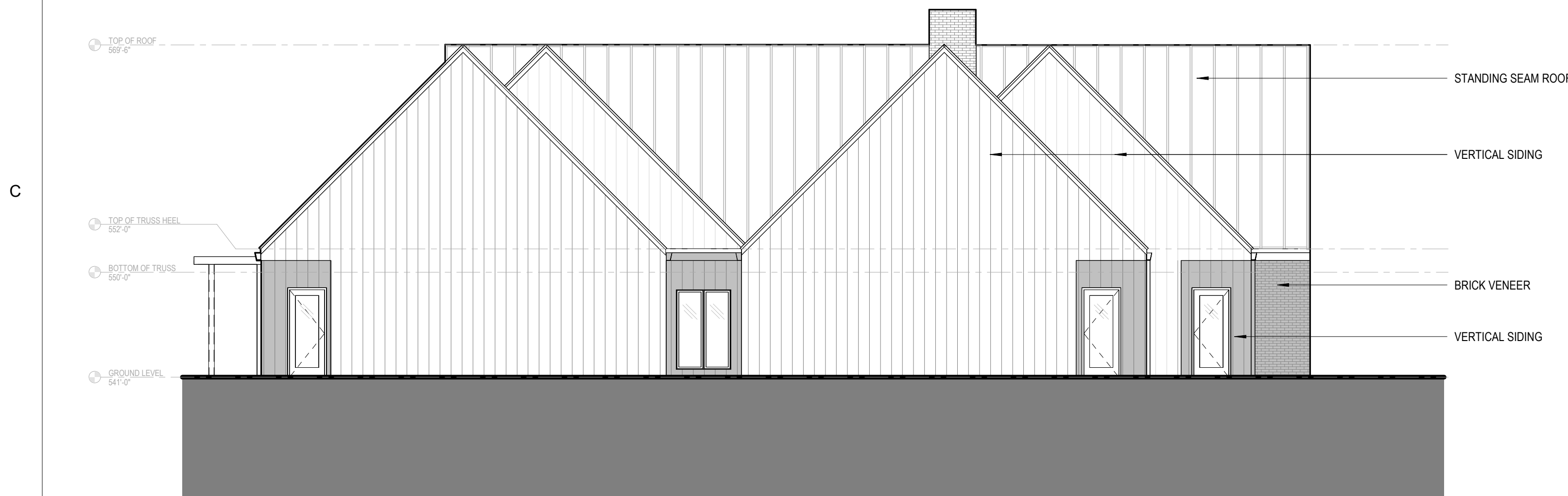
C1 WEST BUILDING ELEVATION 1/8" = 1'-0"
